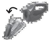
4. Put the filter back into the filter housing and place filter assembly back into the dirt cup. Reassemble dirt cup to body, align bottom first and rotate up until it clicks.
