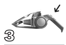
PRESS THE HANDLE RELEASE BUTTON TO PIVOT HANDLE FOR EASY CLEANING.
