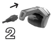
PLUG IN & CHARGE UNIT UNTIL THE CHARGE INDICATOR LIGHT GOES OUT (CHARGING MAY TAKE UP TO 4 HOURS).
